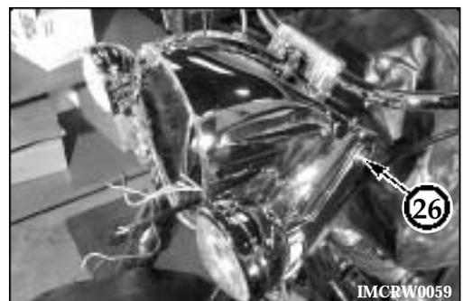
28 From inside the headlamp housing, use a 5/16" socket to remove the three nuts and washers securing the headlamp spear mounted on the top of the housing.
