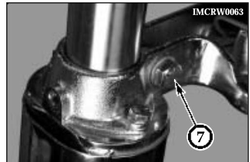
11 Tighten the stem crown nut to 40-45 foot-pounds and bend the tab washer against the face of the nut.
