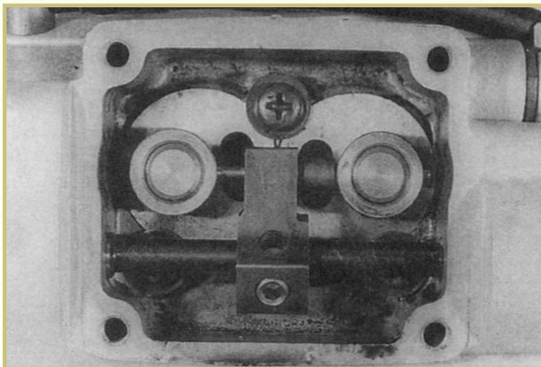
*Note:* The figure shows the power valve used on a Suzuki RM 125.
