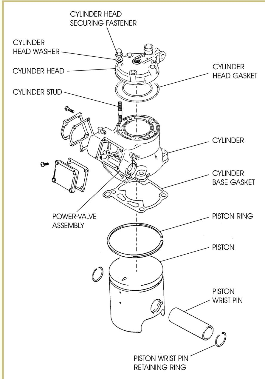
Figure 2 shows an exploded view of the top-end assembly of an air-cooled two-stroke engine.
