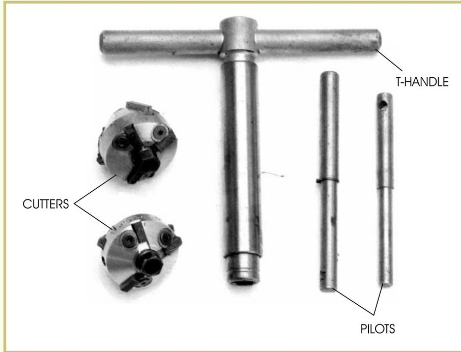
**FIGURE 24—Placement of a Valve Seat Cutting Tool** (Courtesy of American Suzuki Motor Corporation)
