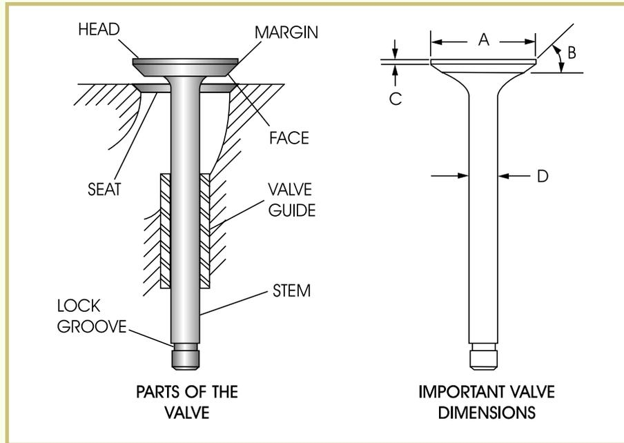
Valves must operate under a variety of extreme conditions. As a result, certain areas of the valve assembly often show signs of wear or physical damage. Because they're located in the combustion chamber, valves can reach temperatures of well over 1,000 degrees Fahrenheit under normal operating conditions! It's not surprising that they can actually begin to melt under these high temperatures. Heat tends to wear away the exposed surfaces, particularly the valve heads.
