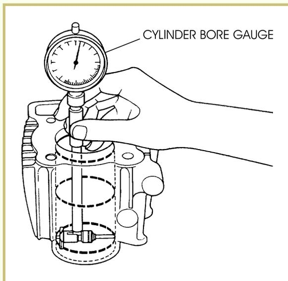
Insert the cylinder bore gauge at a point near the top of the cylinder and take a reading of the micrometer. The gauge is then moved to a point near the center of the cylinder and a reading is taken there as well. Finally, the gauge is positioned at the bottom of the cylinder and another reading is taken. This is done for both the X and Y axis measurements to determine the cylinder's trueness (Figure 10). The readings are compared and the difference indicates the amount of wear.
