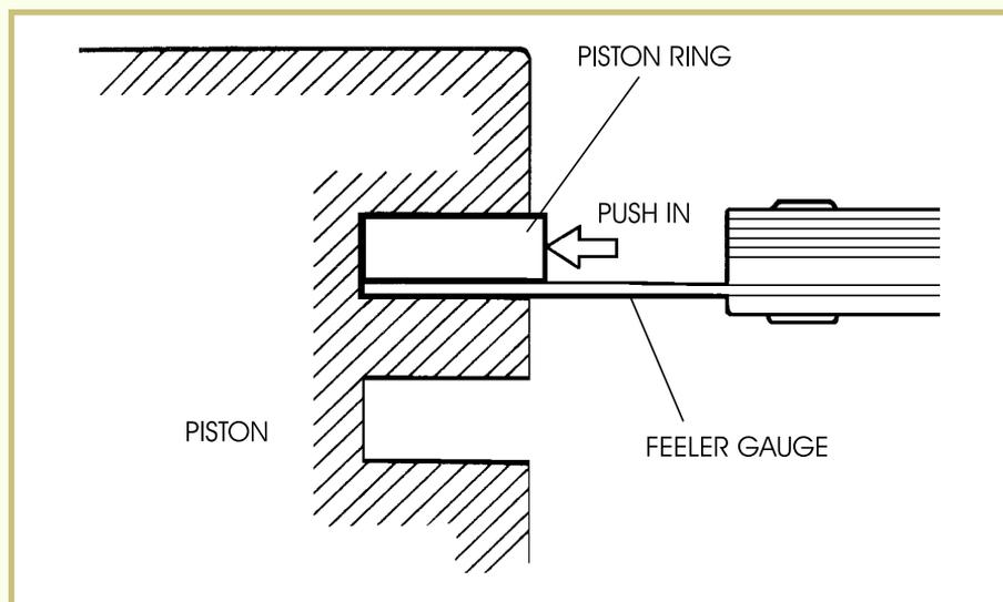
Note that because a small amount of clearance should always be present, a ring tips slightly under normal operating conditions, as shown in [Figure 7](#). As the piston goes down the cylinder during the intake stroke, the ring tips and scrapes excess oil off the cylinder wall. During the compression and exhaust strokes, the piston rises and the tipped ring glides over the oil film remaining on the cylinder wall.
