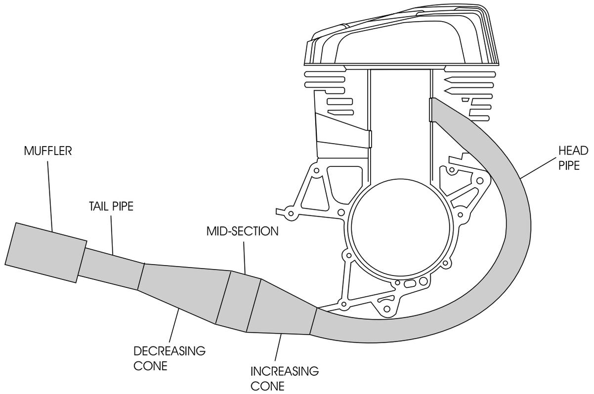
**FIGURE 7—Expansion Chamber Used with a Two-Stroke Engine** (Courtesy of American Suzuki Motor Corporation)
