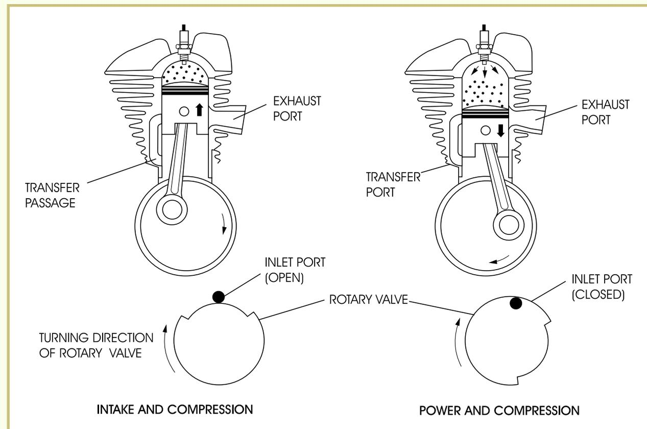
**FIGURE 18**—This illustration shows a rotary-valve two-stroke induction system. (Image courtesy of Yamaha Motor Corporation, U.S.A.)
