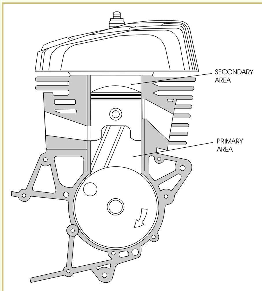
Two-stroke engines have different types of ports to allow for the flow of intake and exhaust gases.
