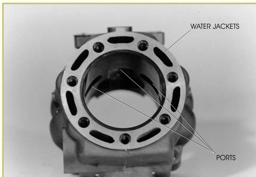
The ports in a two-stroke cylinder may be *bridged*. Bridged ports are used on very wide ports to prevent the piston ring from catching on the edge of the port. Both the upper and lower edges of the ports are *chamfered*. When ports are chamfered, the sharp edge of the port is removed to help keep the piston ring from catching as it moves up and down in the cylinder.
