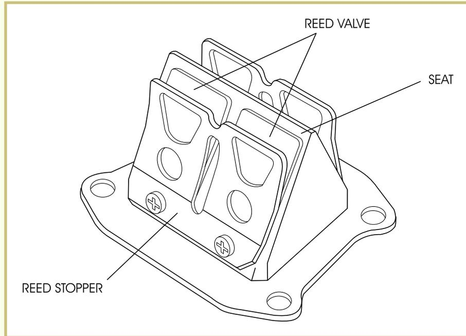
The piston of a reed valve engine has either a cutaway or holes on the intake side of the piston skirt to allow the flow of the intake mixture at all possible times (Figure 14). Reed valves are made from one of two materials: stainless steel or fiber resin material (fiberglass or carbon fiber). There are different types of reed valve induction systems used on motorcycle and ATV two-stroke engines.
