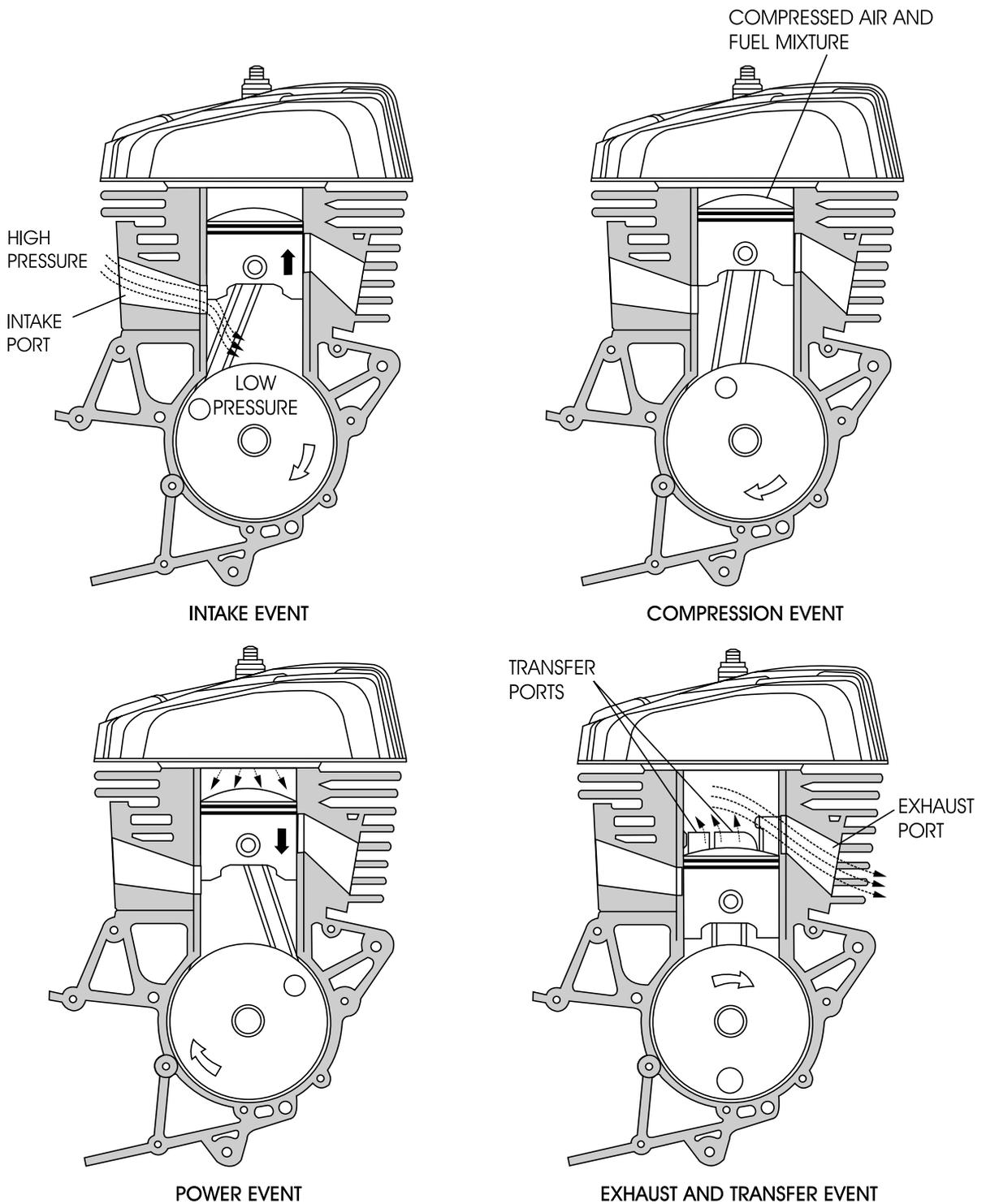
**FIGURE 11**—This illustration shows the five events that occur in one crankshaft revolution on a two-stroke engine. (Courtesy of American Suzuki Motor Corporation)
