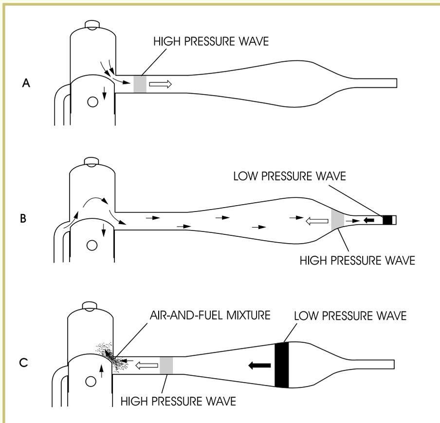
The remainder of the high-pressure wave travels out the tailpipe and is exhausted to the atmosphere. As the wave exits the tailpipe, it creates a low-pressure wave that moves back up the tailpipe behind the reflected high-pressure wave. The low-pressure wave is timed to arrive at the exhaust port to draw or scavenge the exhaust gases after the next power stroke. The expansion chamber must be properly tuned to permit the pressure waves to cause the desired effect.
