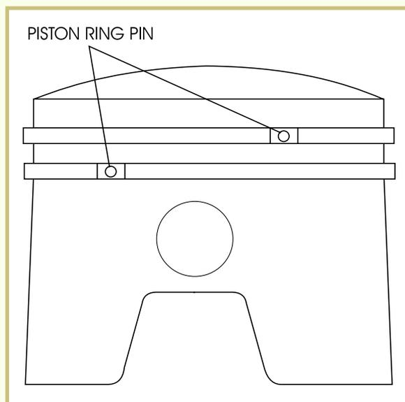
**FIGURE 4—The Parts of a Typical Two-Stroke Piston**
