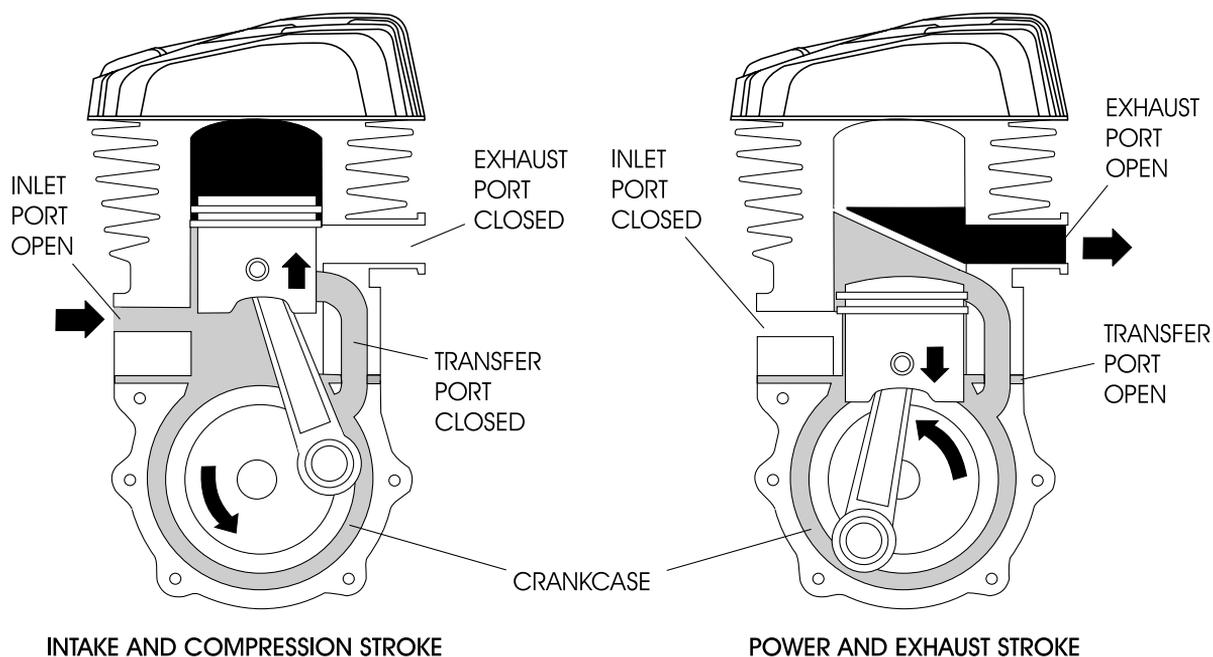
**FIGURE 8**—In a two-stroke engine, as the piston moves upward, it completes the intake and compression stages of operation. As the piston moves downward, it completes the power and exhaust stages of operation.
