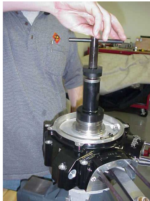
FIGURE 1.5 shows seals being set with special Jim's Tool
