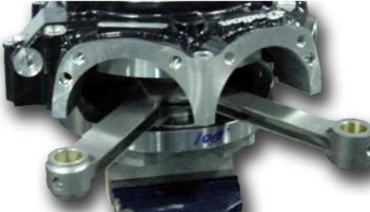
FIGURE 1.2 shows the connecting rods, male to the right and in their respective cylinder paths.
